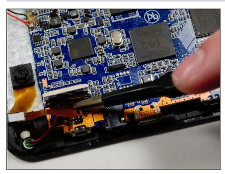
Using a pair of the Precision Tweezers, remove the ribbon wire from the clip.
