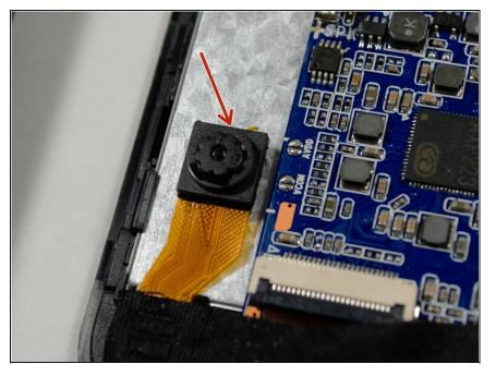
Gently dislodge the camera using the Metal Spudger. The camera is now ready to be replaced.
