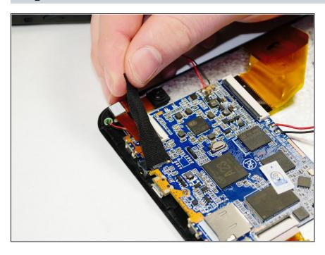
Carefully remove the black electrical tape connecting the motherboard to the ribbon wire.
