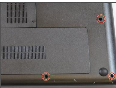
With all the screws removed from the previous guides. Remove the final eight M2.5X5 mm Philips screws on the back of the laptop
