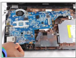
Unlatch the final cable and gently remove the Motherboard.
