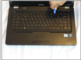
Open up the front of the laptop. Use a plastic opening tool to carefully pry open the keyboard from the edges.
