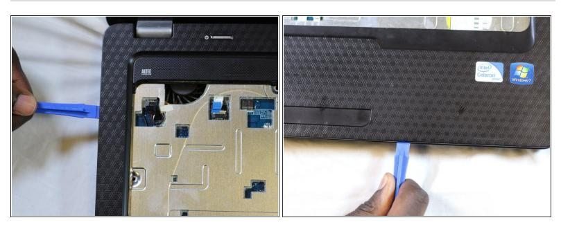
Using a plastic opening tool to lift the sides of the cover.
