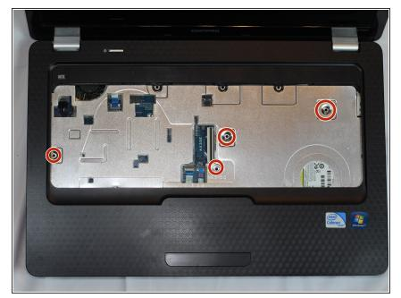
Remove the four M2.5x5 mm Phillips screws from the exposed keyboard cover.
