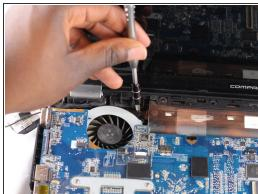
Remove the three M2.25x5 mm Phillips screws.
