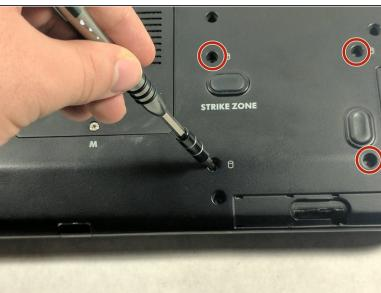
Unscrew the four Phillips head screws on the back of the computer.
