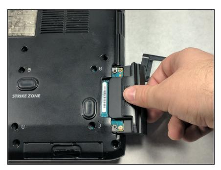
Pull the piece that protruded out slightly in the last step away from the computer to remove the hard drive.
