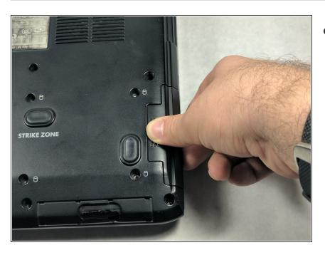
Press the small black button on the side of the computer. There should be a piece that slightly pops out when this is done.
