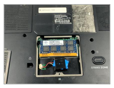
Lift off the panel the screws were holding.
