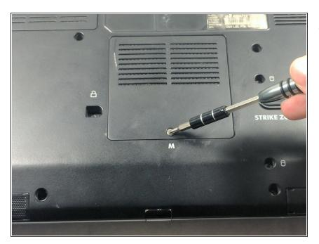
Unscrew the Phillips head screw on the back of the computer.
