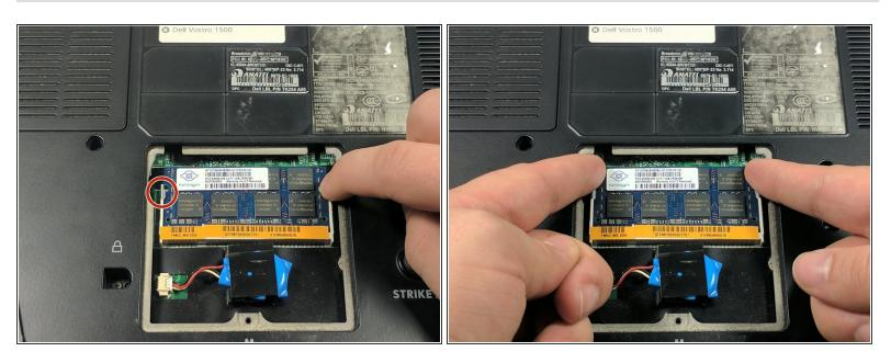
Push the two tabs at the sides of the RAM towards the sides of the computer.
