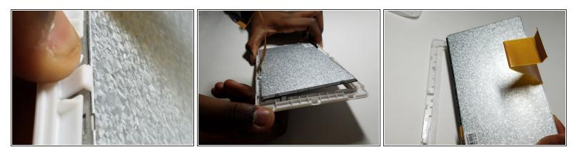
• Slowly remove the screen component off the tablet by clipping the screen from the tablet outine
