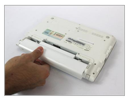
Slide the battery out of its housing.
