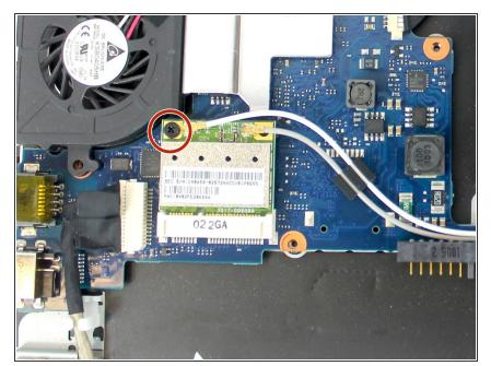
Remove the 3.5 mm Philips #1 screw.
