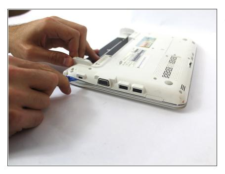
Carefully insert the plastic opening tool in the seam between the lower casing and the chrome bezel.
