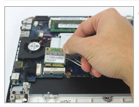
Gently remove the wireless card from its socket.
