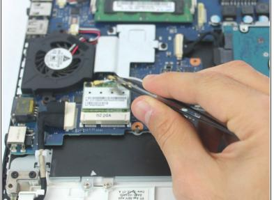
• Carefully with tweezers, lift both connectors to disconnect them from the wireless card.
