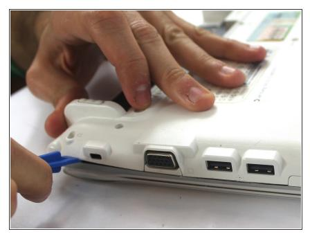
Slide the opening tool across all sides of the lower case, and lift it up to remove the case and reveal the internal components.
