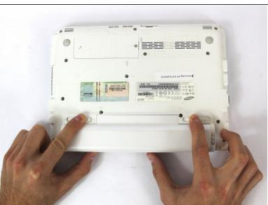
Carefully slide both locking pins to the unlocked position.
