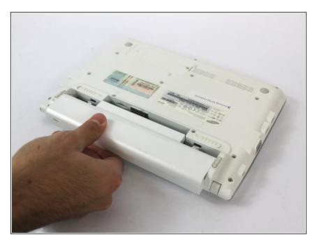
Slide the battery out of its housing.
