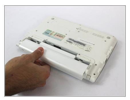
• Slide the battery out of its housing.
