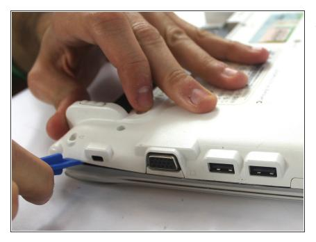
Slide the opening tool across all sides of the lower case. Then, lift it up to remove the case and reveal the internal components.
