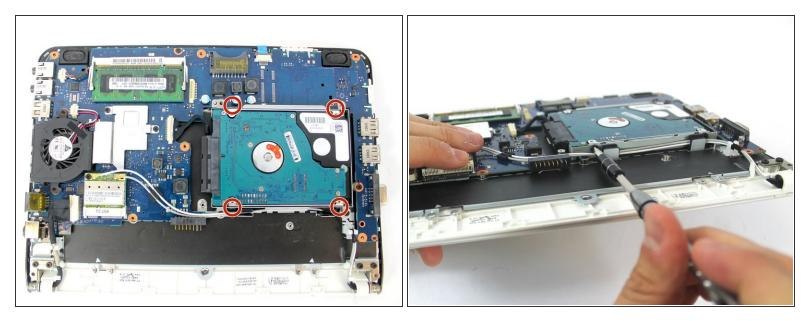
• Remove the four black 3.5 mm Philips #1 screws on the (side) of the hard drive.
