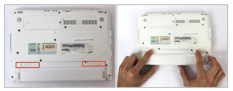
• Carefully slide both locking pins to the unlocked position.
