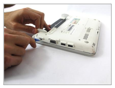
• Carefully insert the plastic opening tool into the seam between the lower casing and the chrome bezel.
