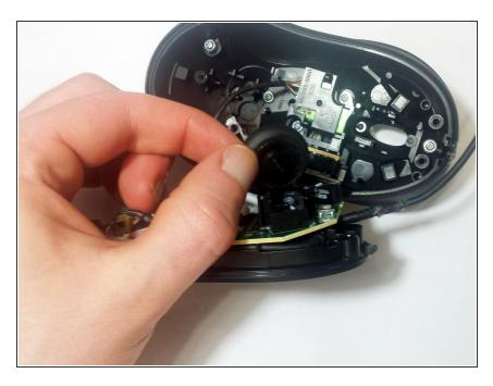
Simply lift the scroll wheel out of the compartment it sits in. It can then be cleaned or replaced as desired.
