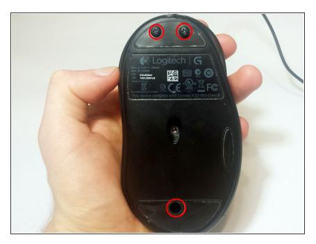
Use a Phillips #1 screwdriver to remove the three 5 mm Philips screws on the bottom surface.
