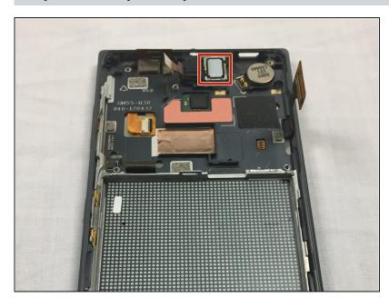
The speaker is located at the top of the device to the right of the headphone jack.
