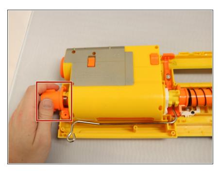
Now that the cover is off and the screws are out, pry off the barrel of the device.
