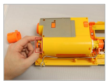
Once the orange barrel of the device has been pried off, proceed to take the metal clip off from where it is currently located.
