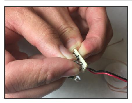
Next, the last step is to gently remove the LED light from the circuit board and replace the bad LED light bulb with a new one as shown below.
