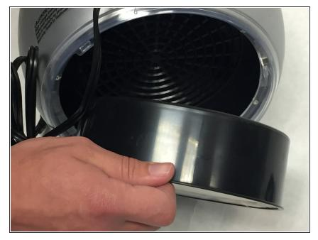
Grab the edge of the filter housing and pull the filter away from the rest of the device.
