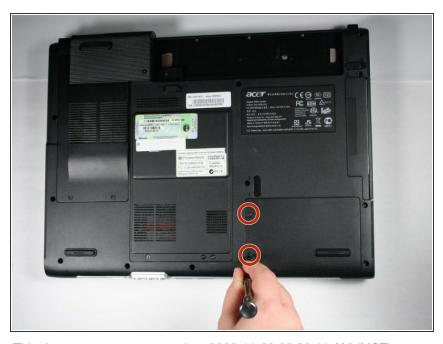
Unscrew the two 4.6 mm Phillips #1 screws on the left side of the hard drive panel in the lower right corner on the back of the laptop using the phillips head j1 bit.
