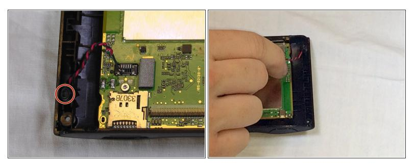
• Use your hands to grab the wires, and gently pull the microphone up and out of the casing.
