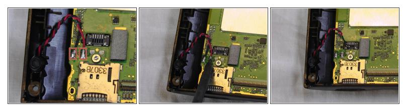
• Use your soldering iron to disconnect the wires from the motherboard. Disconnect the ground wire (the black one) and the positive wire (the red one).
