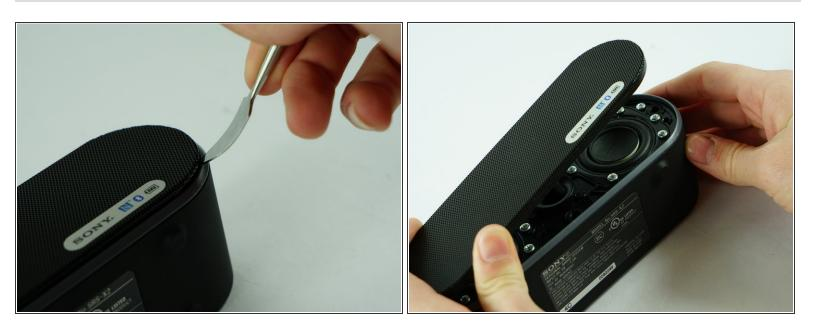
Use the metal spudger to pry the face screen open. Pull away from the device to remove.
