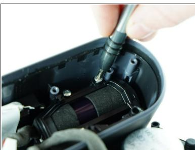
Remove the four, 11 mm, Phillips#1 screws on the battery cover plate.
