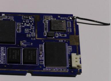
Remove the plug from the motherboard socket.
