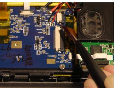
Remove the wire belt from the socket.
