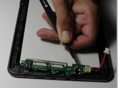
Use the plastic removal tool to pry the audio PCB and pull away from the frame to remove it.
