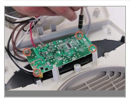
Remove four 12mm Phillips #2 screws from the circuit board.
