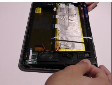
Use the plastic removal tool to remove the plastic frame.
