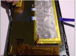
Using the plastic removal tool, lift the LED screen from the battery side, and use the tweezers to help lift the LED screen upwards.
