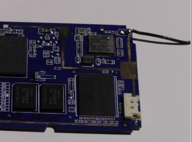
Remove the plug from the motherboard socket.
