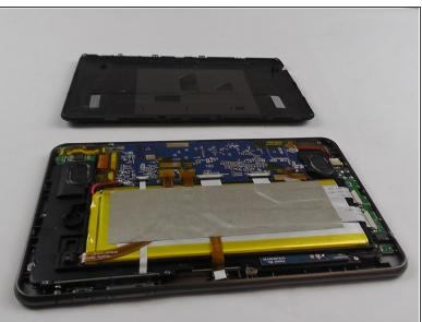
Once the back panel has been pried away from the bottom and sides of the Neo3DO, lift the back panel up and away from the tablet.
