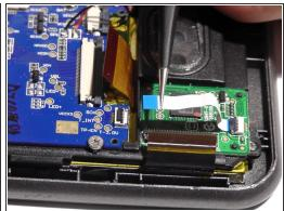
Lift the black tab and then remove the wire belt.
