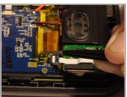
Remove all the tape attached to the motherboard.
