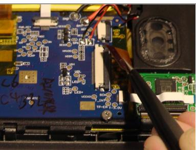
Remove the wire belt from the socket.
