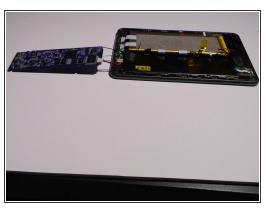
• Use the flat end of the plastic spudger to remove the motherboard and turn it underside-up.
