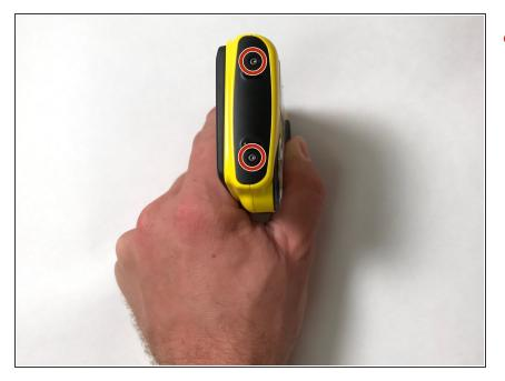
Using a H1.3 hex head bit, remove the two 2mm screws on the side of the camera.
