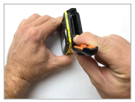
Release the battery from its secured position by pulling the orange tab back. The battery can then be removed from its compartment.
