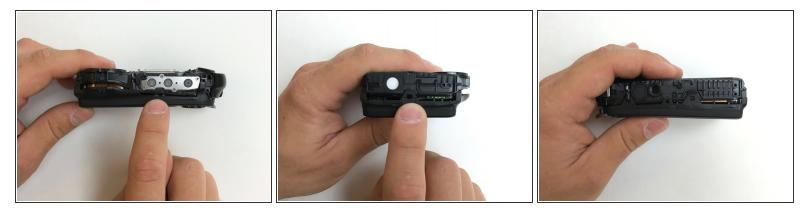
• Unclip the front interior panel from the top, bottom and side of the camera.
