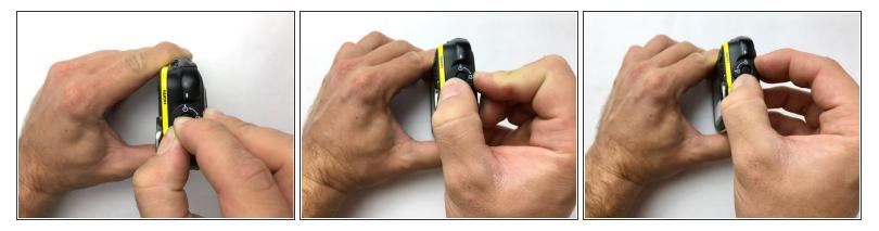
• Open the side panel which houses the battery compartment. Press the center button down and twist the dial.
