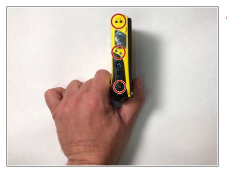
Using a Phillips PH000 bit, remove the five 2mm screws on the bottom of the camera.
