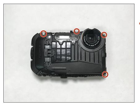
Using the H1.3 hex head bit, remove the four screws on the front of the camera.
