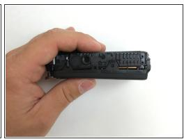
Unclip the front interior panel from the top, bottom and side of the camera.
