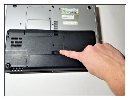
Slide the battery release latch to the right and hold in place.
