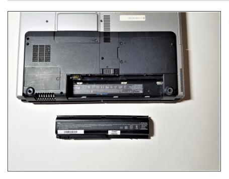
Lift the front edge of the battery up and remove it from the compartment.
