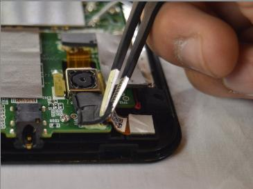
• Use <u>tweezers</u> to remove the black foam stickers from the front facing camera to expose the wiring.
