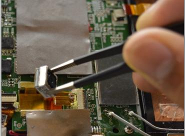
• Using tweezers, lift the camera out from system board.
