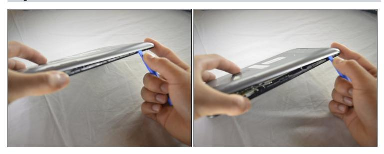
• Slide the tool around the perimeter of the tablet until the edge of the cover is completely separated from the display panel assembly.
