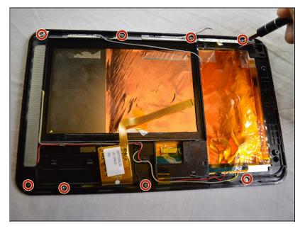
Unscrew 8 screw using a Phillips 00 screwdriver.
