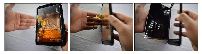
• Remove the screen by holding the tablet in one hand with the back of the LCD screen facing up. Slowly rotate the tablet so the screen falls into your other hand.
