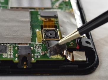
• Use the <u>tweezers</u> to remove the black foam stickers from the rear facing camera to expose the wiring.
