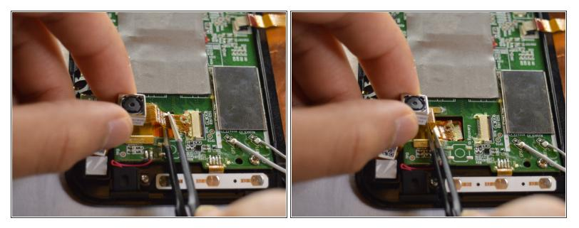
Use tweezers to pull the wire out from the connector. Pull away from the connector, parallel to the tablet.
