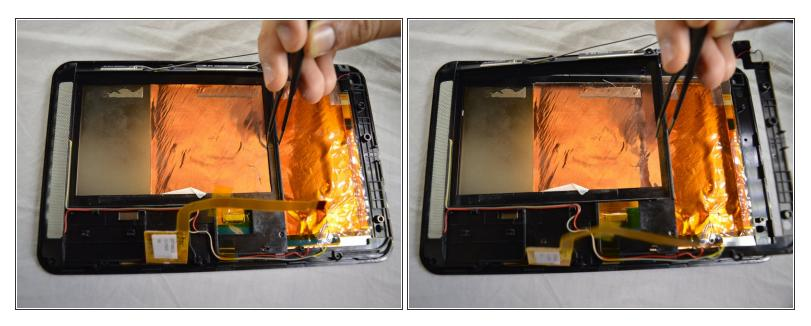
• Grab the center of the plastic frame, which has the speaker, and lift to remove it.
