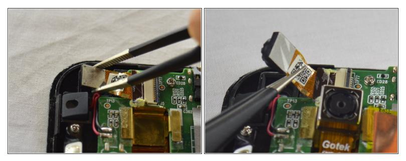
• Lift the camera out from system board and firmly pull the wire out from the connector.
