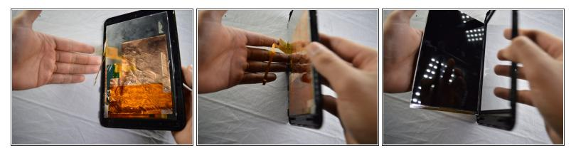
• Remove the screen by holding the tablet in one hand with the back of the LCD screen facing up. Slowly rotate the tablet so the screen falls into your other hand.
