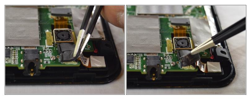
Use the tweezers to remove the black foam stickers from the rear facing camera to expose the wiring.
