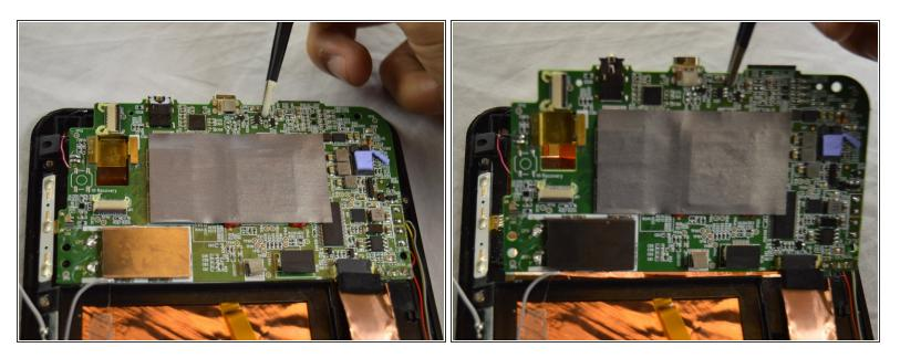
• Using tweezers, lift the system board and remove it.
