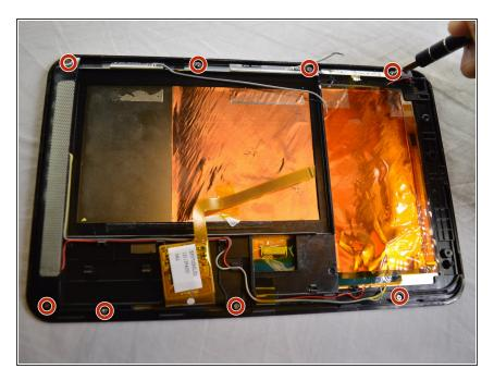
Unscrew 8 screw using a Phillips 00 screwdriver.
