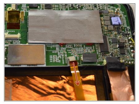
• Disconnect the LCD wire from the connector by pulling away from the connector, parallel to the tablet.
