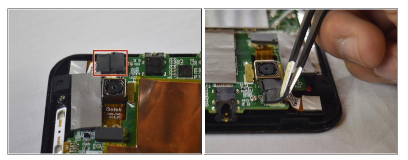
• Use tweezers to remove the black foam stickers from the front facing camera to expose the wiring.
