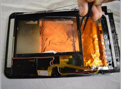
• Grab the center of the plastic frame, which has the speaker, and lift to remove it.
