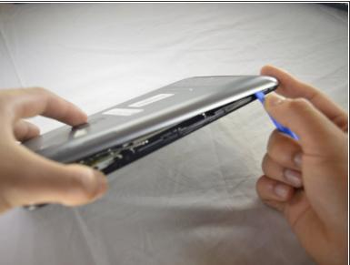
Slide the tool around the perimeter of the tablet until the edge of the cover is completely separated from the display panel assembly.
