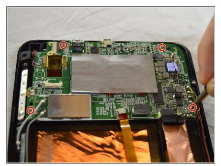
Remove the four screws from the motherboard using a Phillips 00 screwdriver.
