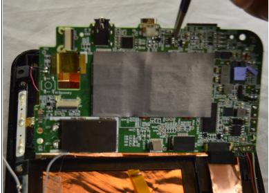
Using tweezers, lift the system board and remove it.
