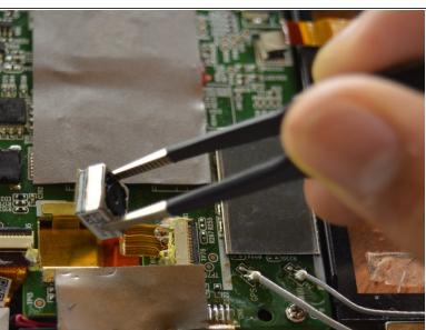
Using tweezers, lift the camera out from system board.
