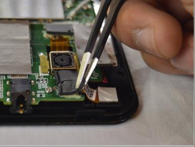
Use tweezers to remove the black foam stickers from the front facing camera to expose the wiring.
