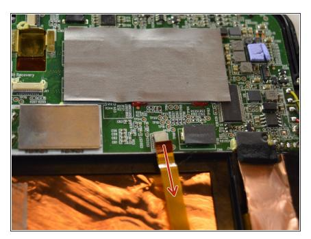
Disconnect the LCD wire from the connector by pulling away from the connector, parallel to the tablet.
