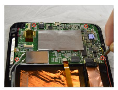
Remove the four screws from the motherboard using a Phillips 00 screwdriver.
