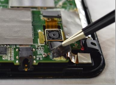
Use the tweezers to remove the black foam stickers from the rear facing camera to expose the wiring.
