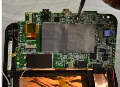
Using tweezers, lift the system board and remove it.
