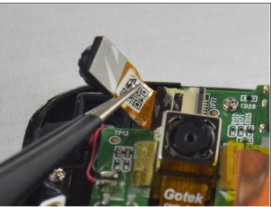
Lift the camera out from system board and firmly pull the wire out from the connector.
