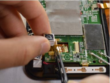
Use tweezers to pull the wire out from the connector. Pull away from the connector, parallel to the tablet.
