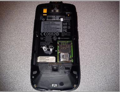
(i) Take the battery cover and battery out of the device and put the unit on its front.
