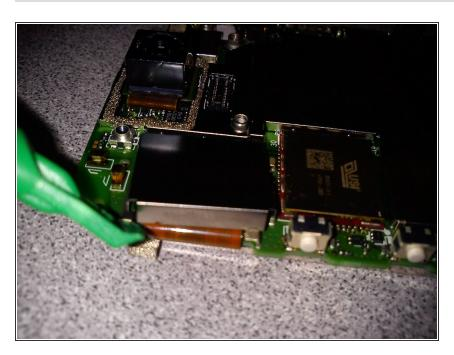
Pry off metal cap to remove shielding to access LCD flex cable.
