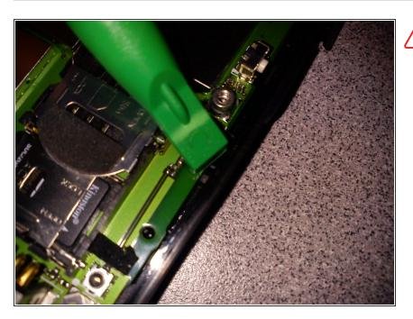
After all the fingers and clips have been released/removed, use a plastic prying tool to carefully pry the logic board out of the frame.
