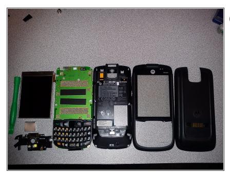
Lay all the parts out so you can easily see what needs replacing or repairing.
