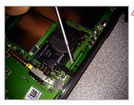
Near the memory card slot on the right side carefully lift the logic board over the finger to release the logic board from the frame.
