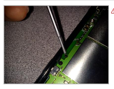
On the left side carefully lift the logic board over the finger to release the logic board from the frame.
