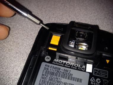
Remove a total of 6 T5 torx screws
