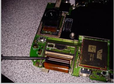
• Use a flat head screwdriver to flip up the FPC connector.
