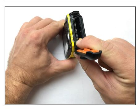
Release the battery from its secured position by pulling the orange tab back. The battery can then be removed from its compartment.
