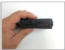
Unclip the front interior panel from the top, bottom and side of the camera.
