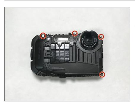
Using the H1.3 hex head bit, remove the four screws on the front of the camera.
