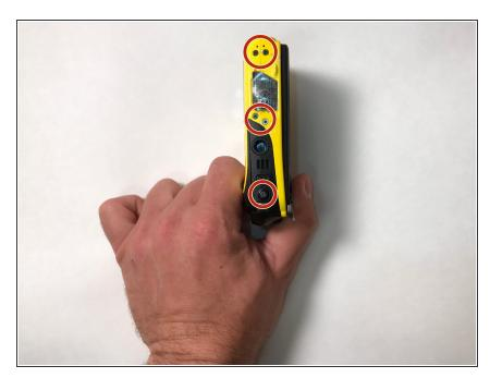
Using a Phillips PH000 bit, remove the five 2mm screws on the bottom of the camera.
