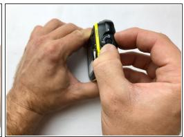
Open the side panel which houses the battery compartment. Press the center button down and twist the dial.
