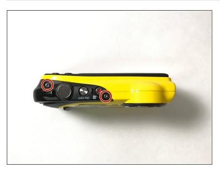
Using a H1.3 hex head bit, remove the two 2mm screws from the top of the camera.
