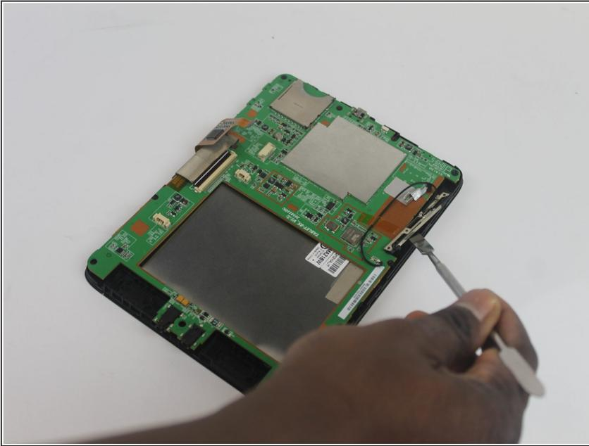
**⚠** This guide shows the use of incorrect tools. Always use ESD safe tools when dealing with delicate internal components.
