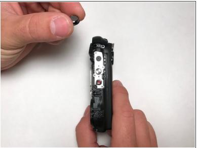
Once the exterior case is removed, separate the plastic depressor to ensure there is nothing lodged in or around the button, preventing proper functionality. To reassemble your device, follow these instructions in reverse order.
