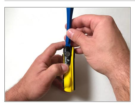
Using a plastic opening tool, gently pry up the edge of the button case, located at the top of the camera, until it unclips.
