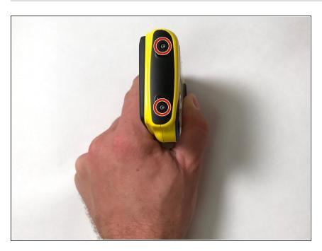
Using a H1.3 hex head bit, remove the two 2mm screws on the side of the camera.
