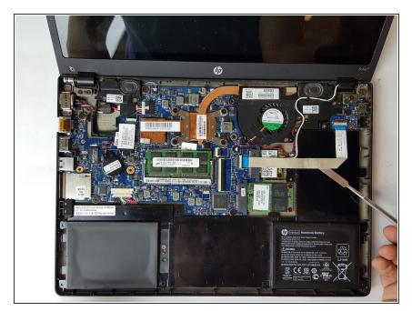
Separate the ribbon from the battery by wedging the flat metal spudger between the two.
