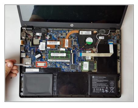
Remove the motherboard connection using the nylon spudger or your fingers.
