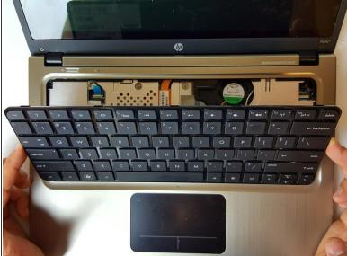
Slide the keyboard up and towards the screen just enough to separate the keyboard from the top cover.
