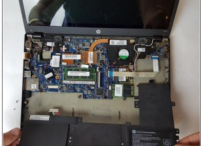
Remove old battery and replace with a new one.
