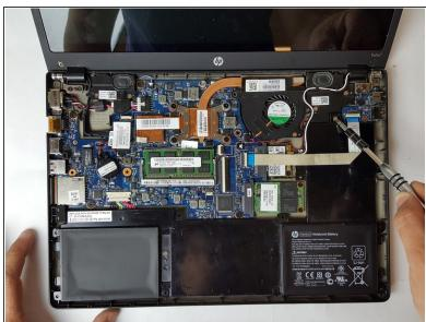
• Use a PH1 screw head to remove the two, 3mm screws.
