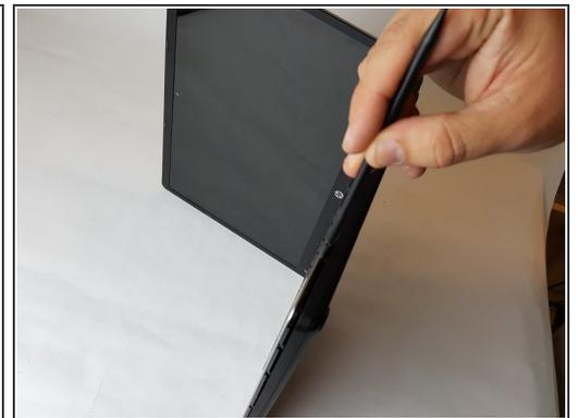
**i** This step requires unlocking the very fragile plastic clips along the frame; take care not to damage them.
