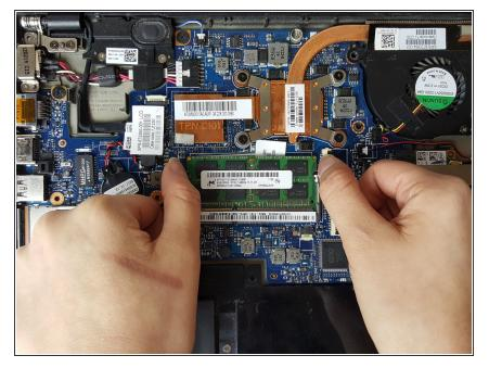
Using the tips of your fingers, gently apply opposite outward force until the two clips are no longer holding the RAM stick.
