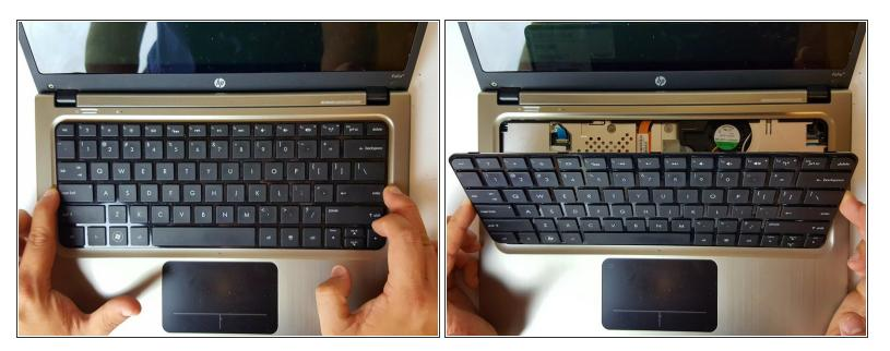
Slide the keyboard up and towards the screen just enough to separate the keyboard from the top cover.
