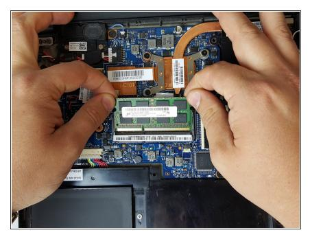
• Carefully remove the old RAM by sliding it towards the screen.
