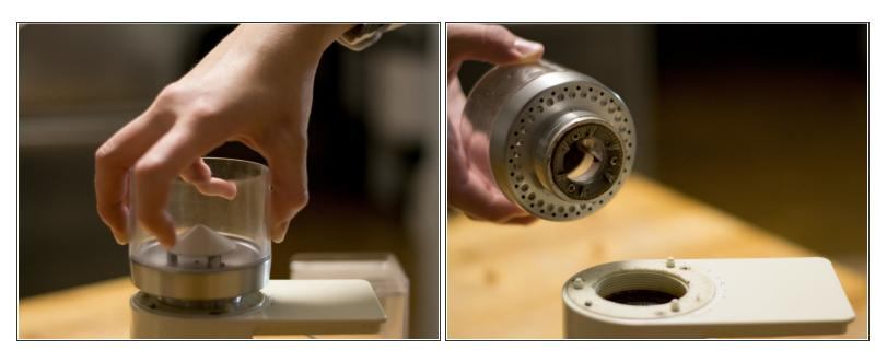
Now it's time to rotate the bean container anti-clockwise to remove it from the machine
