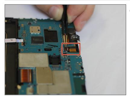
i The front camera is located at the top, middle of the motherboard. The red rectangle in the image to the left depicts its location.
