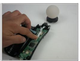
Cautiously remove the circular white piece at the top without removing the LED inside.
