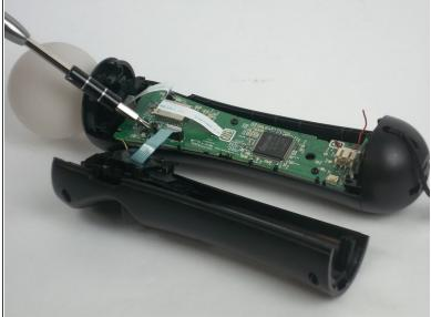
Remove the two 1.2mm Phillips #1 screws.
