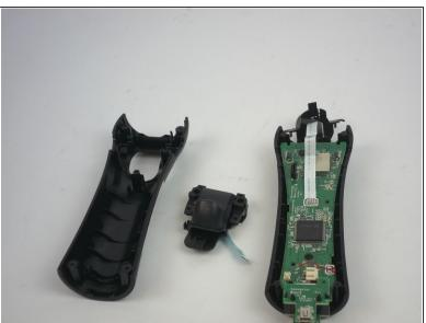
Remove the trigger button from the controller.
