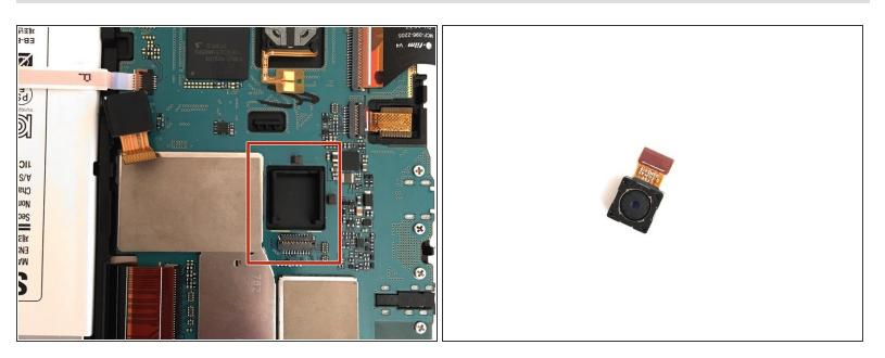
• The picture illustrates what the device should look like once the back camera is removed.
