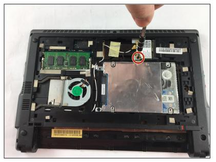
Using a Phillips #0 screwdriver, remove the indicated M2x2mm screw.
