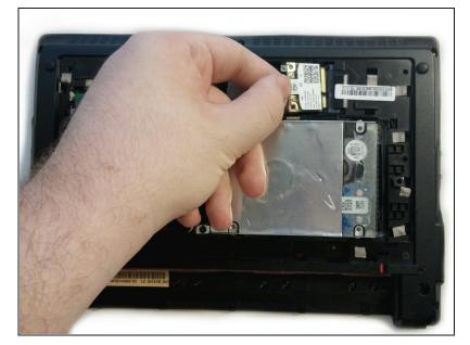
Grasp the sides of the wireless card and slide it out of the port.
