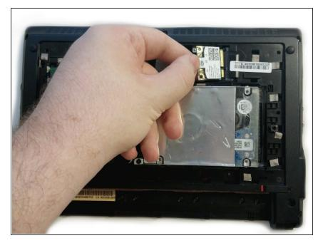
Grasp the sides of the wireless card and slide it out of the port.
