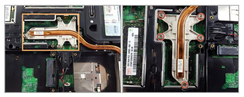
• The system's heatsink is the copper pipe and large metal assembly held down by five screws.
