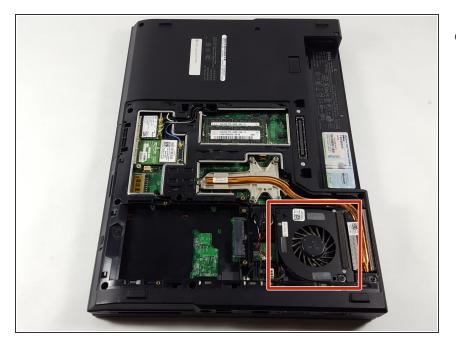
• The cooling fan is located near the edge of the device, on the side with the vent, and is contained within a plastic shroud.
