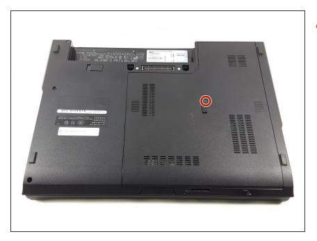
Unscrew the single 3.5mm Phillips #1 screw that holds on the bottom plate of the device.
