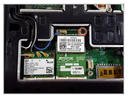
• Unscrew the 4mm Phillips #1 screw that secure the card in place.
