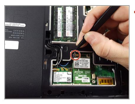
Remove the wire connecting the card to the laptop with a pair of tweezers.
