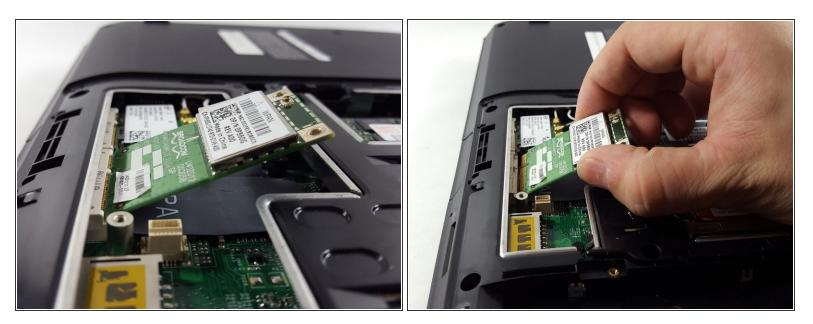
(i) After completing steps 4 & 5, the card will lift up at an angle as shown.
