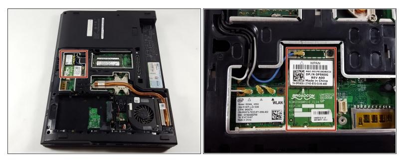
The Bluetooth card is located near the front of the device, and is the expansion card with one antenna attached to it.
