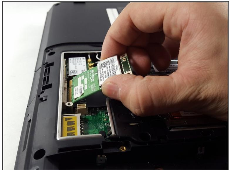
**i** After completing steps 4 & 5, the card will lift up at an angle as shown.
