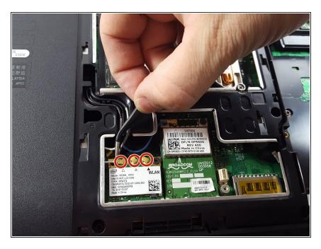
Remove the wires connecting the card to the laptop with a pair of tweezers.
