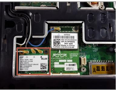
• The wireless card is located near the front of the device, and is the expansion card with three antennas attached to it.
