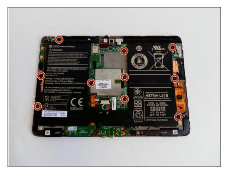
Unscrew the ten 3.3 mm screws securing the battery using a 00 Phillip's head screwdriver.
