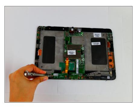
Unscrew the two 3.3 mm screws using a 00 Phillip's head screwdriver.
