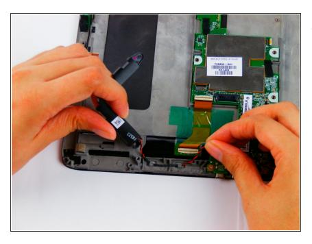
Unhook the left speaker's connector wire to fully remove it from the device.
