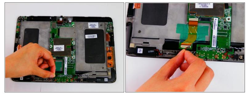
Pull the red and black wire connector up to disconnect it.
