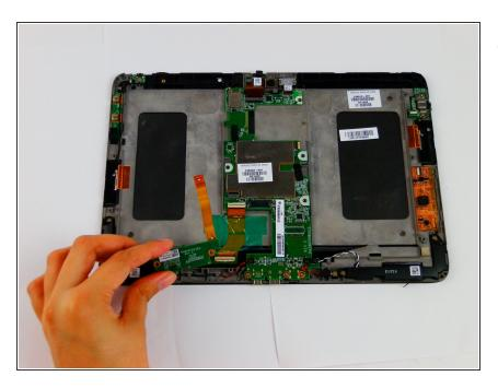
Lift and remove micro card reader board.
