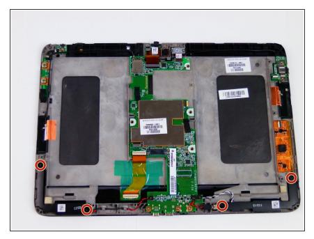
Unscrew the four 3.3 mm screws using a 00 Phillip's head screwdriver.
