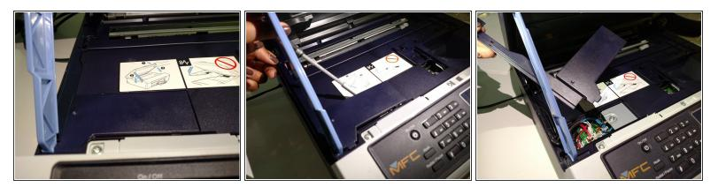
Using a flat head screwdriver, remove the 2nd tabbed panel.
