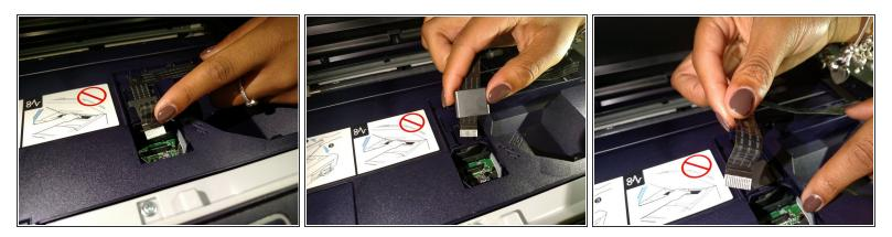
• Gently lift up ribbon cable and pull it through holder then remove ribbon cable from its track.
