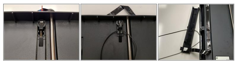
• To remove the belt, first place the image sensor to the side then press down on the gear base to loosen belt and remove from the gear.
