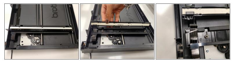
• To remove image sensor, detach the wire strip and pull it out. Remove the two springs that are under the image sensor after its removal.
