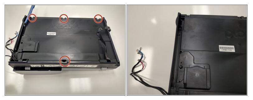
• After removing the scanner assembly, place it on its head. Remove the hinge and 4 screws from the lower scanner portion using Philips-head screwdriver.
