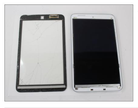
• Lift the touch screen straight up to separate.
