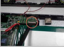
Remove the connection of all of the ribbon cables connected to the motherboard of the device using the Plastic Spudger.
