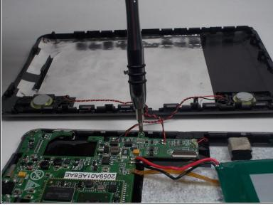
Using the philips head screw driver size PH0, unscrew the screws holding the mother board to the device.
