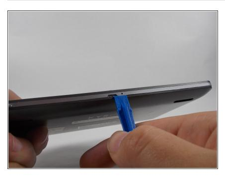
Begin by removing back panel using the large opening tool.
