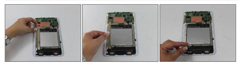
• Lift the white bar on the ZIF connector and pull the metal connector out.
