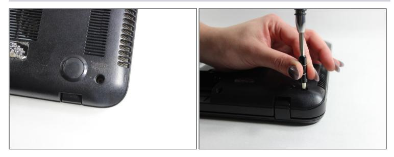
• There are nine 7 mm (5 mm head) screws located around the perimeter of the laptops back panel. Unscrew them all.
