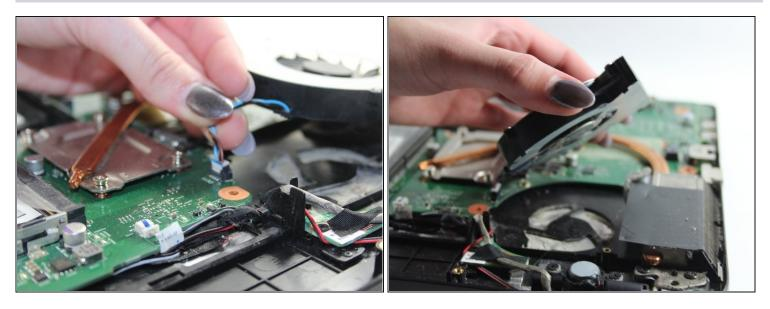
• Unplug the wire located to the left of the fan by pulling gently upwards.
