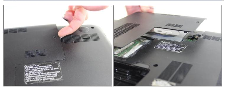
• Once the screw is removed, pry the panel upwards by gripping the groove pictured.
