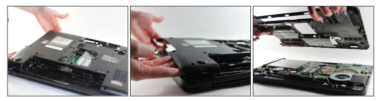
• Get a grip on one edge of the back panel that is now unscrewed and lift its entirety up and away from the device.
