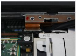
Pry the connectors of the ribbon cables off slowly, lifting straight up. Wiggle gently side to side if necessary.
