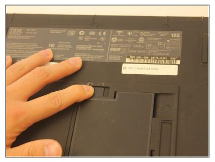
• Move the latch to the side with the unlocked symbol.
