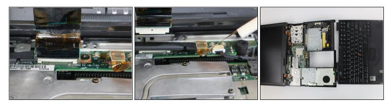
• Pry the connectors of the ribbon cables off slowly, lifting straight up. Wiggle gently side to side if necessary.
