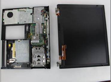
• After you've removed the screws, open the laptop and gently pull the display out.
