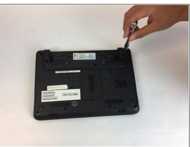
Unscrew three black 1mm screws using the PH1 Phillips-head screwdriver on the bottom of the laptop around the battery.
